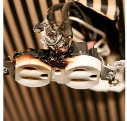
There are several challenges with using aluminum for wiring. Aluminum expands and contracts with current more than copper, which can lead to loose connections at wire terminals that can create arcing and electrical fires.
